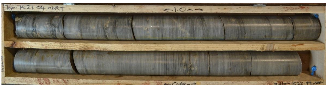
Figure 6-4: Typical example of polyhalite from drillhole SM3a: banding is most visible in the top right of the figure, while the polyhalite in the bottom left is more massive.
